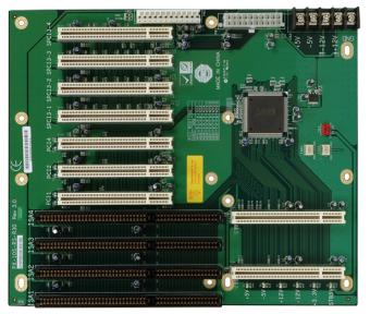
10-slot backplane with seven PCI slots and three ISA slots
